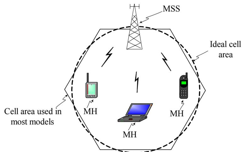
Fig. 1-1. Illustration of a cell with a MSS and mobile hosts (MHs).
