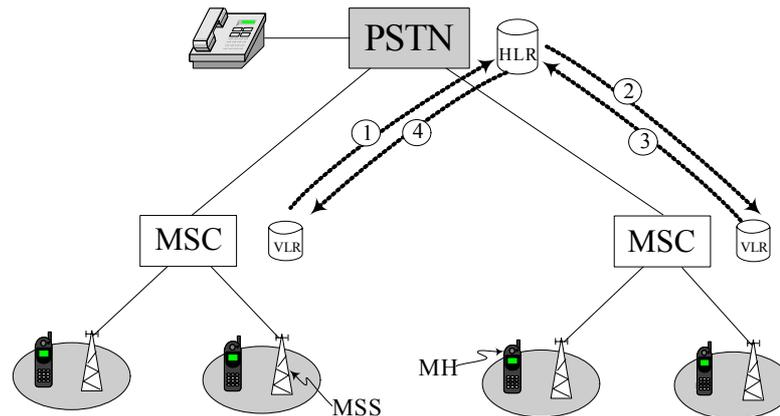
Fig. 1-2. The basic cellular system infrastructure and location tracking scheme.
