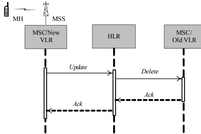
Fig. 1-3. Signal flow of location update for IS-41 scheme.
