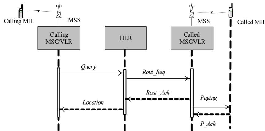
Fig. 1-4. Signal flow of location query for IS-41 scheme.
