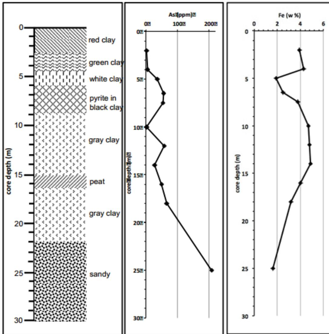
Fig. 4 Core composition, arsenic concentration and percentage of iron with depth
