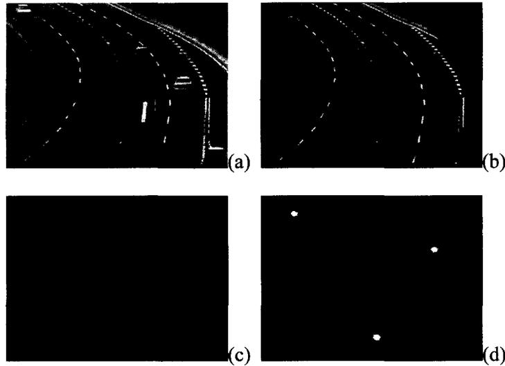
Figure 5. Experiment results for road extraction on different environmental conditions (a) is the input scene, (b) is the daytime results, (c) is the rainy daytime results, and (d) is the nighttime results.
