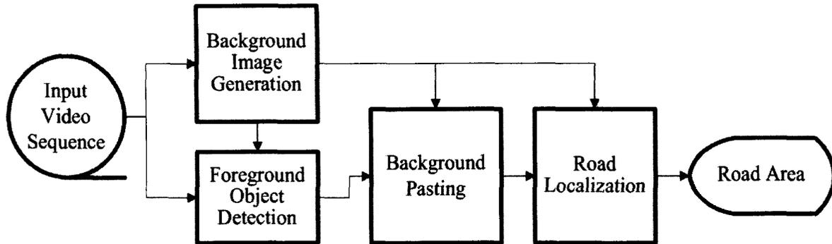
Figure 1. Block diagram for road segmentation.
